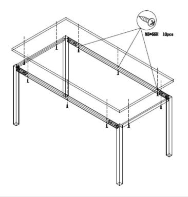
Attach frame to the table top using the provided screws as shown
