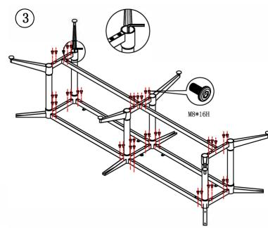
Layout Left, Right and Central Leg Upside Down On a Flat Surface. Slide Central Support Beams Into Legs - Attach Support Beams With M8 Bolts ( Do Not Completely Tighten Bolts) . Once The Frame Is Sitting Flush On the Flat Surface, Tighten All Bolts Completely.
